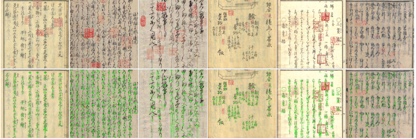
Figure 6. Visualization of the input images (top row) and the recognition results projected onto the corresponding images (bottom row).
